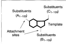
Figure 1. Schematic illustration of a combinatorial library. Each member of the library consists of a common template or scaffold (black) connected via template attachment sites (grey) to different lists of substituents. In this example, there are 100 possible substituents at three sites, leading to a library of 1 million compounds.
